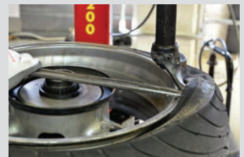
Step 4 : Removing the tyre
